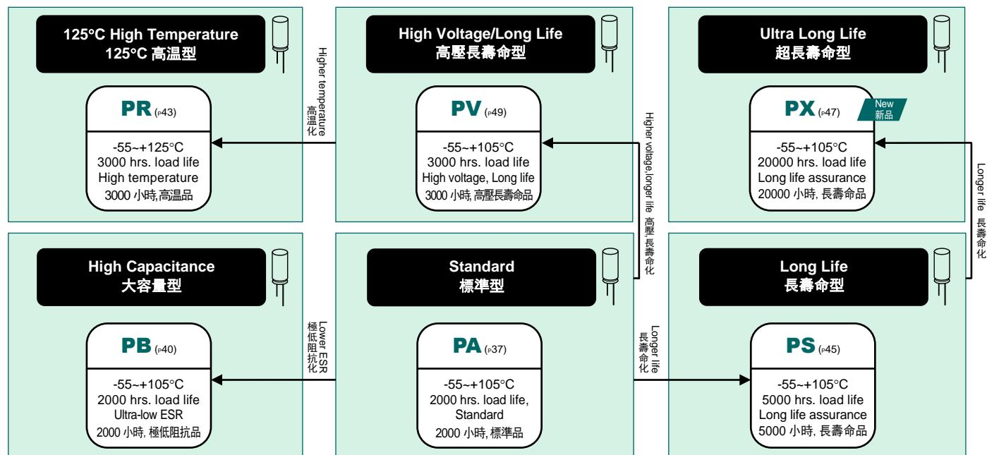
**Conductive Polymer Hybrid Electrolytic Capacitors (Chip & Radial Lead Type) 導電性高分子混合型鋁電解電容器(貼片式及引線式)**
